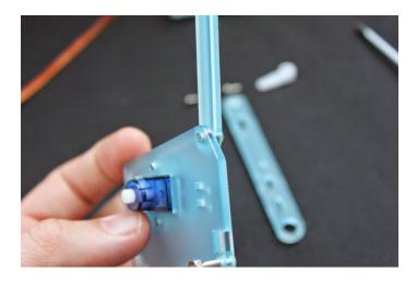
Step 11: Attach to servo and set limits
