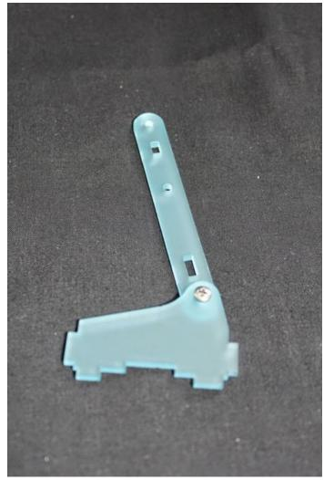
Step 13: Attach the servo horn to the base
